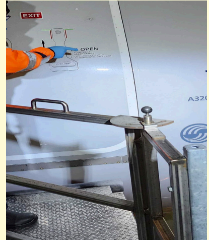
Above: Example of guard rail with a properly secured joint at SFO
