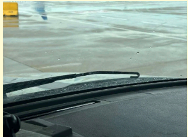
Truck with missing wind shield wiper ORD 6/14/26
