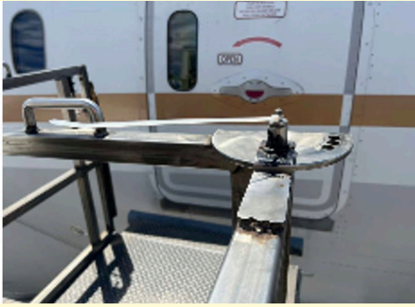
Broken guard rails on two different catering trucks. The left image shows a joint in the guard rail secured with a zip tie, and the center image shows the joint unsecured. ORD 6/15/26 and 6/23/26
