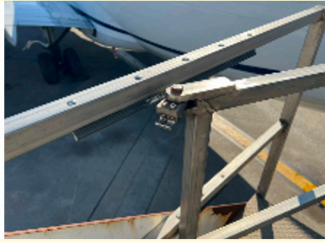
Broken guard rails on two different catering trucks. The left image shows a joint in the guard rail secured with a zip tie, and the center image shows the joint unsecured. ORD 6/15/26 and 6/23/26
